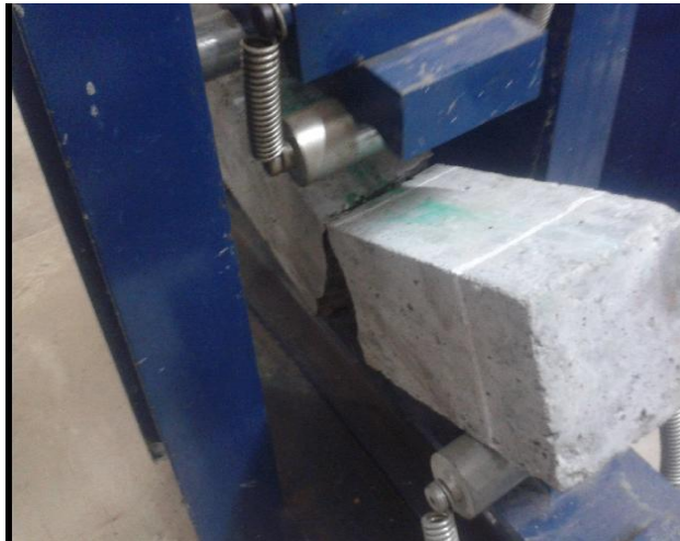
Fig. 3: Flexural strength testing machine
