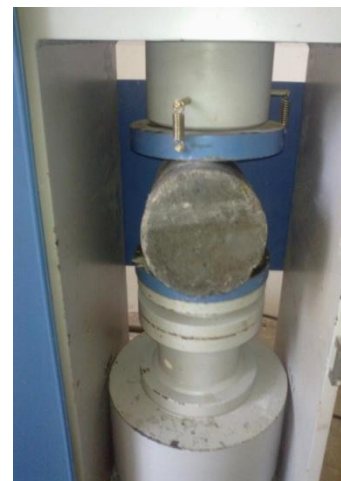
Fig. 2: Split tensile strength testing machine
